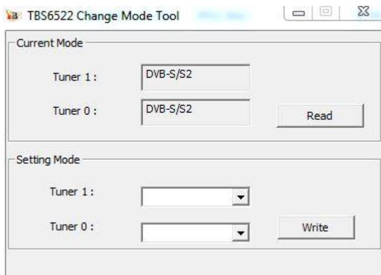
The settings made are saved for further use. If you want to change the saved mode, this is also possible at any time. Proceed as described in the last paragraph. Be sure to connect your TBS-6522 card according to the selected reception mode (example: satellite cable with DVBS /S2).
